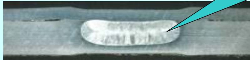
Cross-sectional photograph of weld
