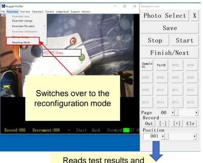
The reconfiguration mode allows you to change or modify existing parameter files.
