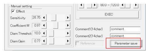
1. Click [Save Parameters] in the bottom right of the [Toolbox] dialog box to overwrite the parameter file.
