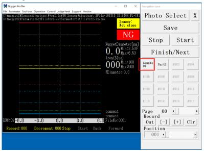
1. Activate Nugget, and in the [Navigation Record] dialog box, click the button to which the component whose parameters are to be modified is registered.
