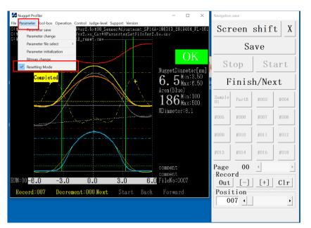
5. Click [Parameter], then [Reconfiguration Mode] in the top left of the screen to terminate the reconfiguration mode.
